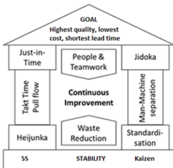
Figure 1. The house of Toyota Production System (adapted from Liker, 2004)
